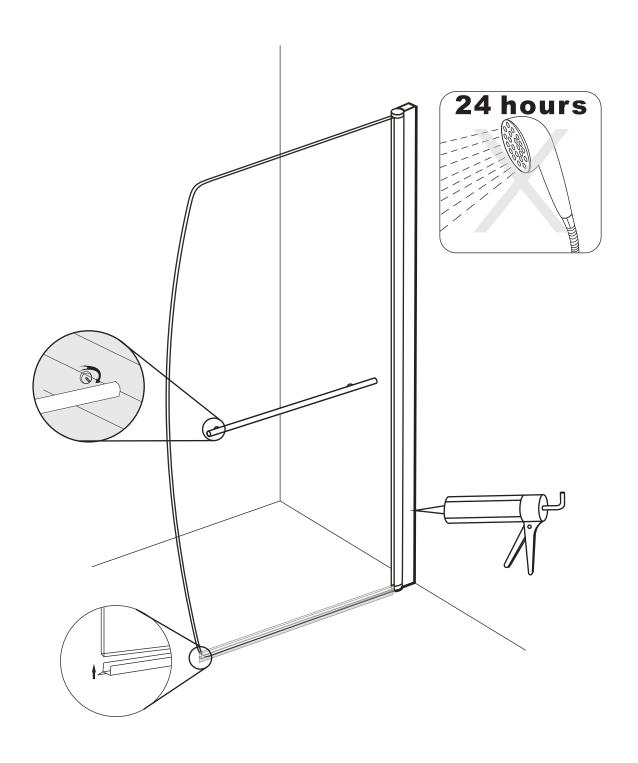
Warning: Don't use the shower enclosure until after at least 24 hours, so that the silica gel can be totally dry.
