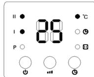
If the room temperature is lower than the temperature shown on the display the appliance stays in stand-by.
