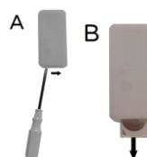
Substitute the battery (following the right polarity) and close the battery slot. For longer inactivity periods please remove the battery.
