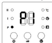
5. Press the button to select the starting time, “00” appears on the display and every time the button is pressed it adds one hour to the starting time.
